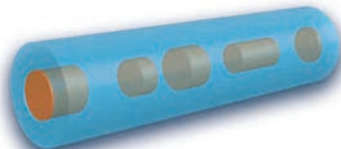
Air pockets and high variance in flux content
