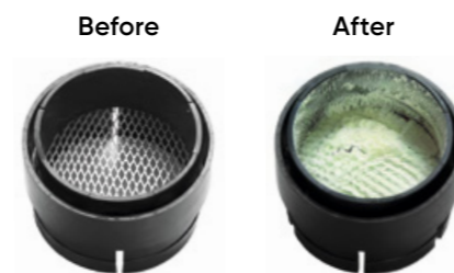
The before/after effect on a small mesh shows the degree of pollution after 90 minutes of soldering.
