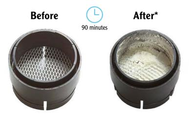
\*Lead free soldering produces up to 250% more particles in the breathing zone than leaded soldering. A clean filter before use and with pollutants after 90 minutes of soldering with lead-free solder wire (3% flux content) shows how effective efficient fume extraction can be and how important fume extraction during soldering is.
