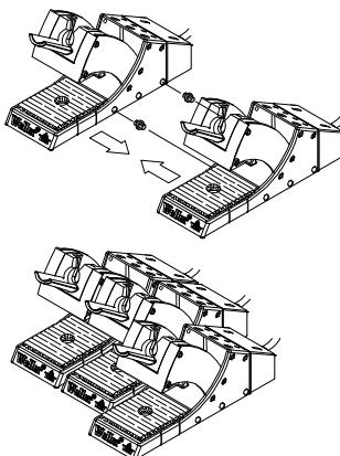
The Weller WDH 10T/20T switching holder, as opposed to a standard safety rest, provides a switching function that can be evaluated by the soldering station. A microswitch integrated in the switching holder is actuated when the soldering tool is deposited or removed.
