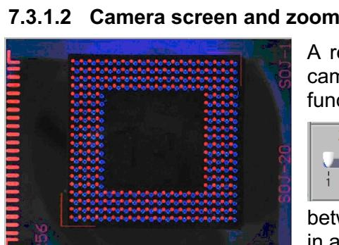
A real-time representation of the camera picture is output in the camera window. Thanks to the high camera resolution, a zoom function is also available with a click of the mouse.
