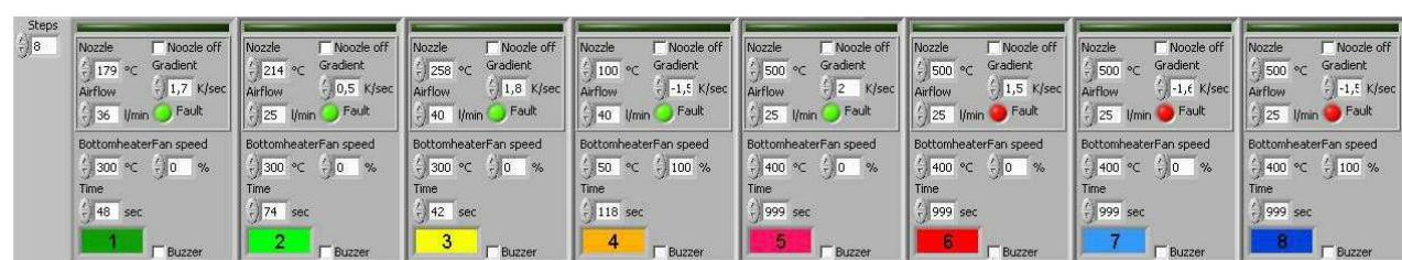
**During application of Gradient mode, operation is always carried out with nozzle pre-heating and the nozzle is already lowered above the component prior to process start. Nozzle pre-heating (Standby Nozzle) is therefore always activated.**
