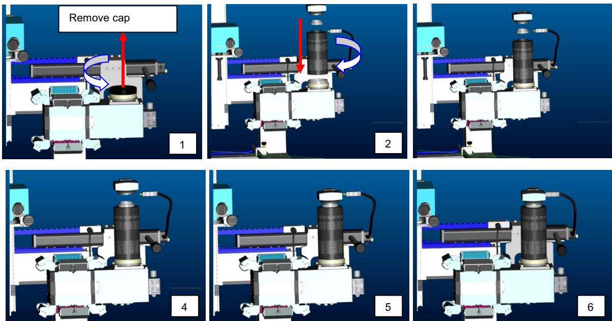
For installation of the 10 x zoom lens, the cover cap on the optical unit housing must be removed. The zoom lens is then assembled as shown in the illustration above.
