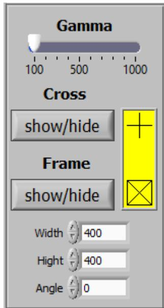
The user can use this button to set an optimised image configuration for the respective requirements, and the Crossing "Show / Hide" or Frame "Show / Hide" buttons are used to display a crosshair or rectangle for easier alignment of components. The size and alignment of the rectangle can be changed using "Width", "Height" and "Angle".
