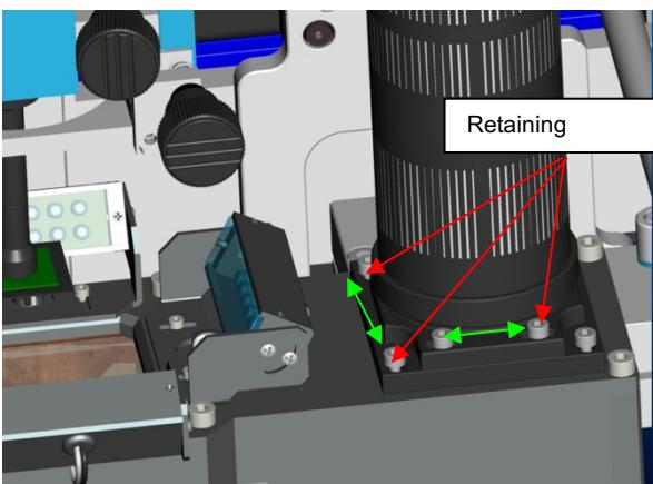
The camera is aligned to the image centre in the factory and has to be checked by fading in the cross-hairs via "Show / Hide" Crossing or the rectangular frame via "Show / Hide" Frame (see chapter 7.3.1.3). In the event of deviations, the camera can be readjusted with the aid of the adjustable camera holder. To do so, release the securing screws on the relevant camera mount level, realign the camera mount and lock it again.
