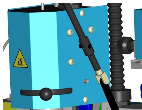
The soldering head is equipped with a rotation-damped articulated lever (16). The soldering head can be lifted off or lowered without vibrations by operating the appropriate articulated lever. A component can also be lifted off during the desoldering process with the vacuum tube when the soldering head is lowered.
