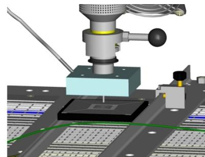
To do so, adjust the depth stop of the soldering head via the knurled screw so that the nozzle when lowered is approx. 0.5 - 1 mm above the template. To align the template precisely, lower the vacuum tube to the template and align the latter precisely.
