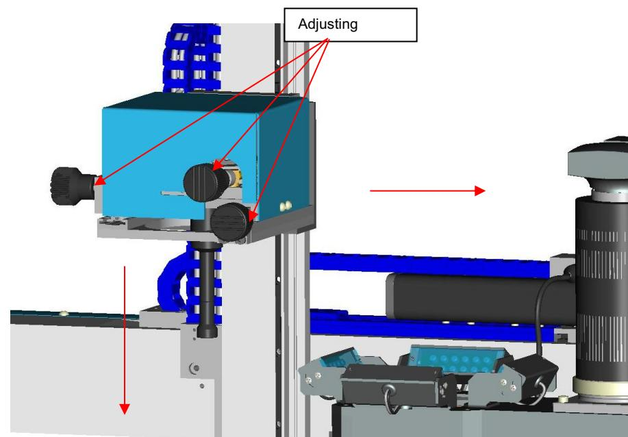
Lift the soldering head off to release the transportation table. Then move the table to "Placement Pos.".
