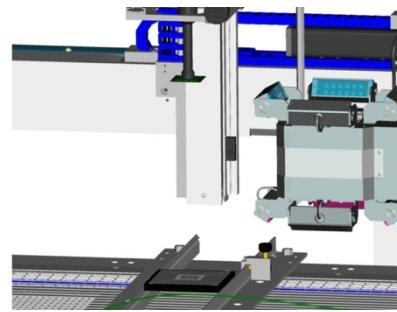
After lifting off, do not alter either the table in X and Y directions or the positioning unit in X, Y and theta directions. Move the split optical unit to the left-hand stop until it engages between the adjustment component and adjustment template and activate the PCB lighting with the positioning software. The adjustment template is shown in red on the monitor. The optimum presentation of the template is achieved using the adjusting rings for the aperture and sharpness.
