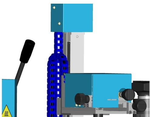
The insertion head is equipped with a stepping motor, which facilitates precise, software-controlled lowering and pick-up of components. Component pick-up with the insertion head (11) is performed with the vacuum nozzle (29). The vacuum is activated via "Vacuum" to lift up components. When lowered, the component can be placed fully automatically with the additional Automatic mode.
