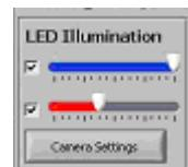
This allows the circuit board or component lighting to be switched on/off and dimmed.
