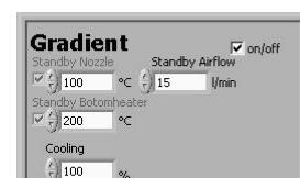
Gradient mode is activated in the Special Functions menu by means of the corresponding option box.
