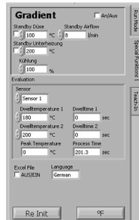
Gradient mode makes targeted heating-up gradients and even targeted cooling down possible. For this purpose, a maximum gradient is specified for each process step.
