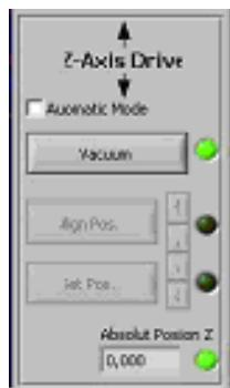
In Automatic mode, automated and partially simplified functions are available to the user. To align the component, the positioning unit can be raised with "Λ" and lowered with "V". The component is lowered with "Set Pos." onto the circuit board. The vacuum is automatically switched off and the positioning unit lifted off.
