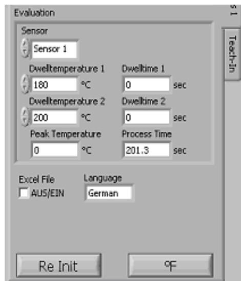
The Re Init button can be used to reinitialise the communication between PC and WQB 4000SOPS without a software restart. Interrupted processes must be RESTARTED.
