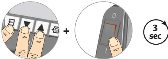
When switching on: Press and hold Exit, UP and DOWN for three seconds
