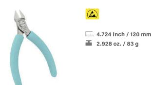
The jaws of the cutter have straight edges and taper to a point. This head shape allows access to difficult to reach areas but reduces the cutting capacity in comparison to the same size oval head cutter.
