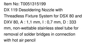
Weller nozzles are constructed to remove all kinds of solder at the solder joint. They are heated and melt the solder. After activating the vacuum the solder is extracted via the integrated tube into the collector.
