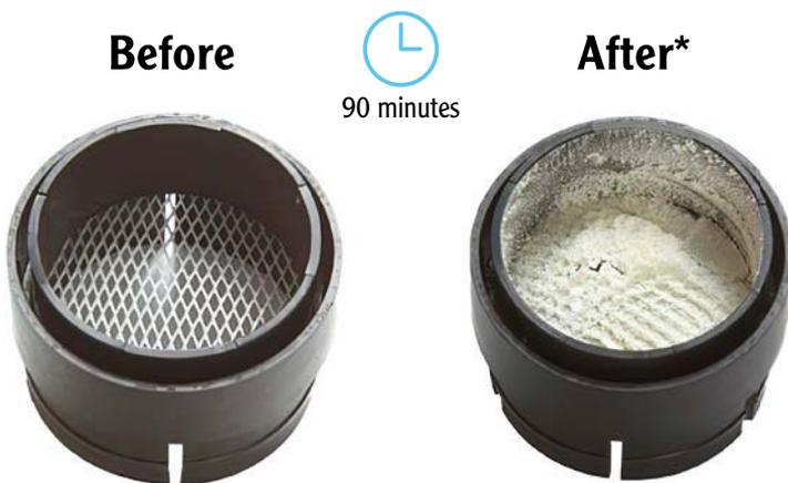
\*Lead free soldering produces up to 250% more particles in the breathing zone than leaded soldering. A clean filter before use and with pollutants after 90 minutes of soldering with lead-free solder wire (3% flux content) shows how effective efficient fume extraction can be and how important fume extraction during soldering is.
